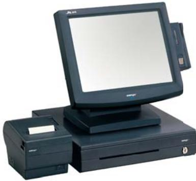
JIVA Bundle: JIVA 5815 / 5715, AURA thermal receipt printer, cash drawer, SD-100 attachment with Integrated MSR and finger print sensor or iButton identification
